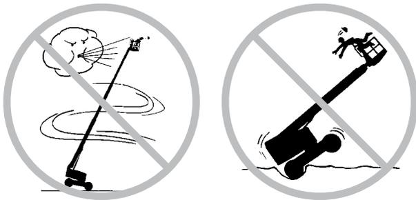
Use extreme care and slow speeds while driving the machine in the stowed position across uneven terrain, debris, unstable or slippery surfaces and near holes and drop-offs.
